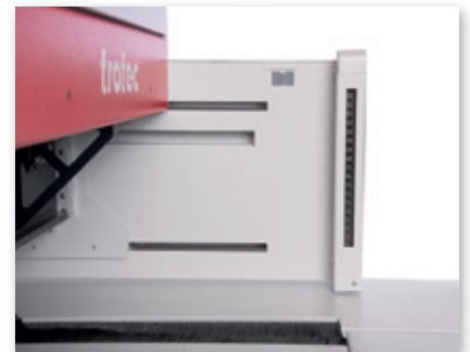
Interlocked safety bumpers with light barriers
