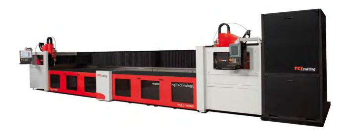
The TCI Cutting SM-M series machine allows both the installation of a second independent cutting table as well as the extension of the main cutting table, thereby maximizing performance.
