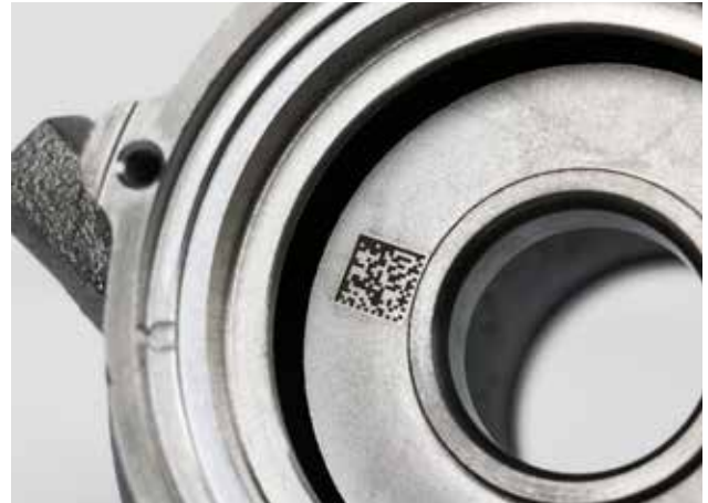
Marking in recesses thanks to long focus distance
