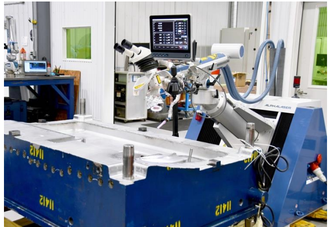
Pulse laser welding mold repair
